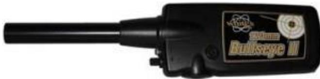
A small pinpoint probe is one of the most useful bits of equipment that you can carry. They are little metal detectors in their own right and their job is to check the inside of your hole, or your pile of dirt, for the target that you are digging. They can save you lots of time and frustration and locate the objects that you would otherwise lose.
